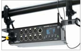
The QolorPIX Tape Controller offers eight ports, each accommodating five meters of tape. It features an integrated power supply, a test function, and flicker finder for easy troubleshooting. It also offers wireless DMX control using City Theatrical's state of the art Multiverse® wireless DMX technology.
